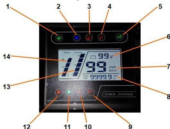
Indicators description: 1, left turning light 2, headlight 3, parking brake 4, reverse gear 5, right turning light 6, battery voltage 7, speed 8, mileage 9, wiper 10 emergency lamp 11, voltage normal 12, under voltage 13, current volume 14, battery volume
