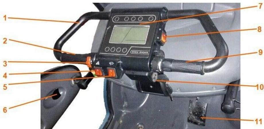
1, Steering wheel 2, Left handle grip 3, Switch of headlight 4, Emergency lamp 5, Wiper switch 6, Door handle 7, Meter board 8, Gearshift switch 9, Right throttle grip 10, Main switch 11, Brake pedal
